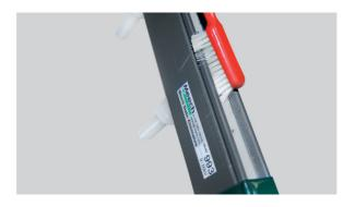
lonising bars will need periodic wiping to clean grey deposits from the surface of the bar. A cloth moistened with a small amount of IPA or methylated spirits is recommended.
