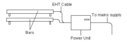
The Power supply converts the primary electricity supply into a high voltage DC output. The generator bars are connected to this output by means of an EHT cable.
