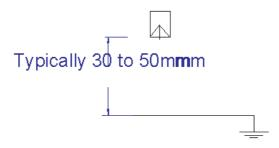
The bar should be positioned away from any other ground reference point. These may disrupt the ion stream and reduce the effectiveness of the bar and the degree of pinning achieved on the process material.
