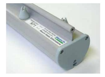
The profile of the Hyperion 971 bar is rounded, with minimal dirt traps, making it useful for cleanroom applications. The bar has good rigidity, allowing it to span wide widths. Mounting is by M4x20 T bolts in a slot at the rear of the bar.
