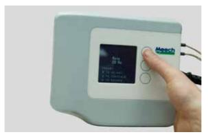
If the bar is positioned a long distance from the target area (600mm-750mm) the "Rate" should be set to the lowest setting. If the bar is positioned close to the target area (150mm -300mm) the "Rate" should be set towards its maximum.
