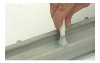
If on inspection, the emitter pins of the Bar are very dirty or damaged they should be replaced. Replacement emitters are available from Meech Static Eliminators Ltd. or your local Meech Distributor.
