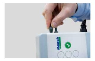
6. Using a high voltage probe (RS 610 281) and meter (RS 610 590) measure the voltage on the pins of the bar. This voltage should be between 3 and 6kV.
