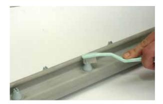
lonising bars will need periodic wiping to clean grey deposits from the surface of the bar. A cloth moistened with a small amount of IPA or methylated spirits is recommended.
