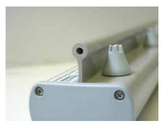
The upstand between the nozzles is a vital feature of the Hyperion 971 bar. By increasing the trucking distance between positive and negative pins, the upstand helps maintain good performance even when the bar is contaminated.
