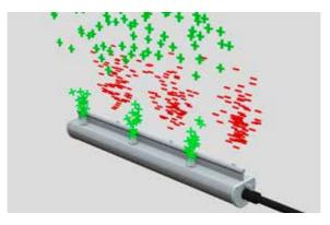
Optimum static elimination can be achieved by adjustment of the "Rate" (frequency of pulsing) and the "Balance" (proportion of positive to negative ions generated) on the Controller.
