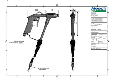
The power unit provides the high voltage ac supply that is required for effective ionisation. The ionising airgun is connected to the power unit by a tough, flexible conduit and high voltage cable. The high voltage is fed to a sharp titanium emitter pin via a safety resistor that renders the pin safe to touch. A corona is generated at the tip of the pin, ionising the surrounding airflow.
