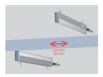
4. The bars must be earthed for correct operation. If in any doubt run an earth wire from the bar to the earth stud on the Power Unit.
