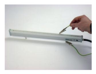
As the pin is approached, a small faint spark should jump from the pin to the wire.
