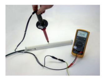
6. If the voltage is below 4.0 kV then the bar should be returned to Meech for service and/or repair.
