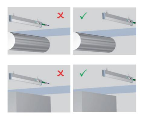
2. Avoid proximity to earthed parts of machinery as this will distort the corona and reduce its efficiency.
