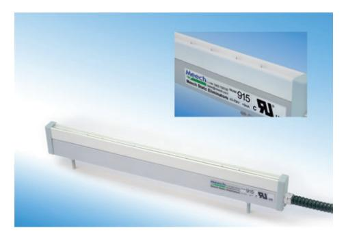
The Meech Model 915 has been designed for use on the most arduous static elimination problems. The special resistive coupling of its emitter pins renders them shockless, whilst giving powerful static neutralisation performance. This enables the bar to eliminate very high static charges on high speed webs and at longer ranges than has previously been possible.
