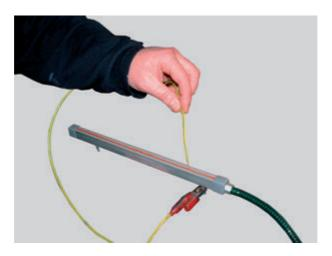
As the pin is approached, a small faint spark sholud jump from the pin to the wire.
