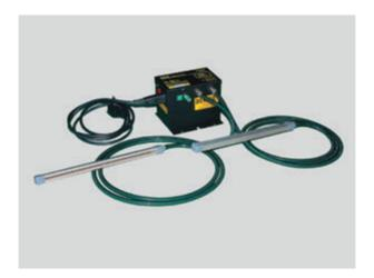
The Power Unit converts the electrical supply into a high voltage, low amperage output. This output energy is transferred to the 914 bar by the HT cable.
