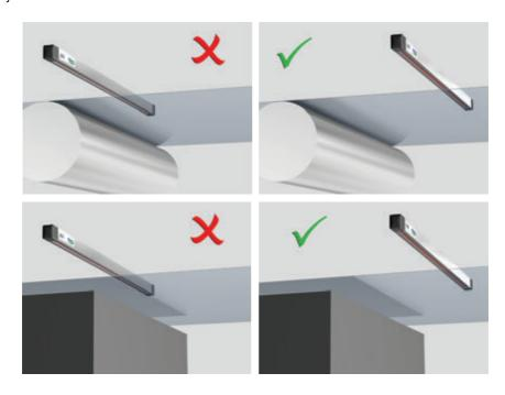
3. Avoid proximity to earthed parts of the machinery as this will distort the corona and reduce its efficiency.
