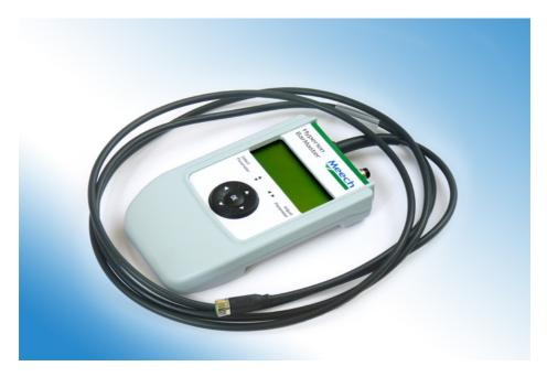
To get the very best performance from Meech Hyperion bars with Integrated Power Supplies, Meech offer the Hyperion BarMaster remote programmer. This unique device is temporarily connected inline with the 24V power supply to the bar and allows adjustment of the output and of the clean-pin alert settings. Once programming is complete the BarMaster is disconnected. When it is re-powered, the Hyperion bar continues to operate at the programmed settings.
