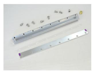
Do not over tighten the M6 bolts and crush the shims. All bolts should be tightened to a maximum of 4Nm or 2.95f/lbs.
