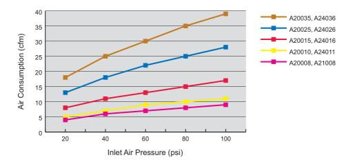
The graph below shows air consumption at varying inlet air pressures.
