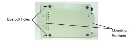
It is also possible to mount the 992v3 (50kV) vertically using the eye bolt holes and mounting bracket provided. (See mounting details at the end of this manual for eye bolt positions). When mounted vertically the front control panel should be removed by unscrewing the 4 retaining screws and refitted as shown in the photos overleaf.
