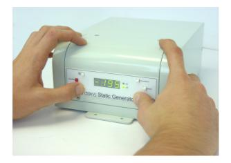
To adjust the current limit (adjustable from 0 -  $260\mu A$ ), press and hold Constant I and use + and - to adjust the current limit. When the Constant I button is released the display will show the actual current being drawn by the system.
