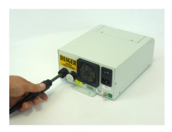
■ Hold the conduit of the generator bar and tighten the fitting by hand until secure.
