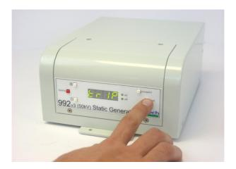
When the 992v3-50kV has tripped, it can also be reset by switching off power to the 992v3-50kV at the mains IEC switch and switching it back on again.
