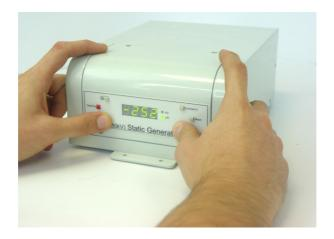
To adjust the current limit (adjustable from  $0 - 500\mu A$ ), press and hold Constant I and use + and - to adjust the current limit. When the Constant I button is released, the display will show the actual current being drawn by the system.
