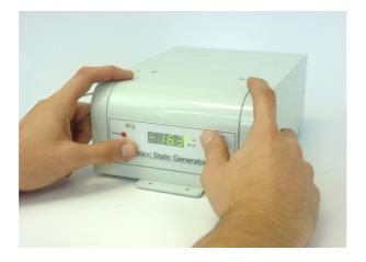
To adjust the output voltage (adjustable from 0 - 30kV), press and hold the Constant V, and use + and - to adjust the set voltage.
