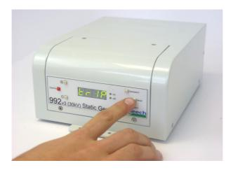
When the 992v3 has tripped, it can also be reset by switching off power to the 992v3 at the mains IEC switch and switching it back on again.
