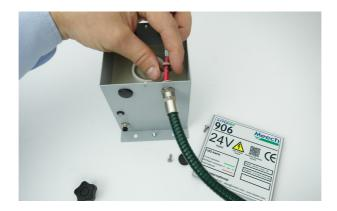
Remove the Black plastic thumb screw and place the appliance cable eyelet over the stud.
