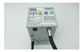
24V 4 pole extension cables are available from Meech in 1, 3 and 8 meter lengths. Ensure the 24V supply is off before connecting the power cable. Once the cable is connected turn the supply back on, the LED's located on either side of the Hyperion power supply should be green. If they are not please refer to the fault finding and diagnostic check located on the next page.
