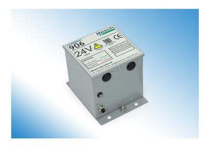
The 24V DC input voltage suits modern machinery and means that they operate independently of local mains voltage and frequency. Settings in the 906 can be adjusted with BarMaster controller. The output voltage can be adjusted from 4kV to 7kV.
