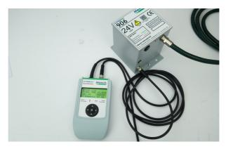
The BarMaster is connected in line with the 906's power supply cable. The power cable is connected to the BarMaster and, in turn, its cable is connected to the Hyperion 906 Unit.
