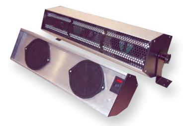
The 935 Ionising Blower provides effective long range ionisation. The Blower comprises an ionisation head and an integrated fan system. A high volume flow of ionised air is generated by blowing air through the ionisation head. Ionisation is provided by powerful 915 Ionising Bars and powered by the 904 Power Supply.
